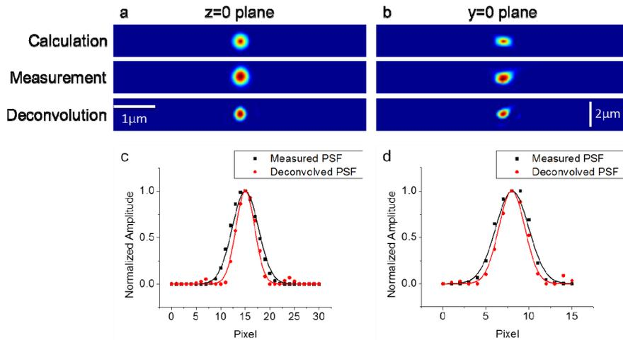
**Figure 1.** Resolution analysis of WDT. (a, b) Transverse and longitudinal cross-sections of the PSF generated from the theory (top), from the measurement of a polystyrene bead smaller than the diffraction spot (middle) and the result of deconvolving the measured PSF with the calculated PSF (bottom). (c, d) Profile along the center of measured and deconvolved PSFs. (Figure adapted from [13])
