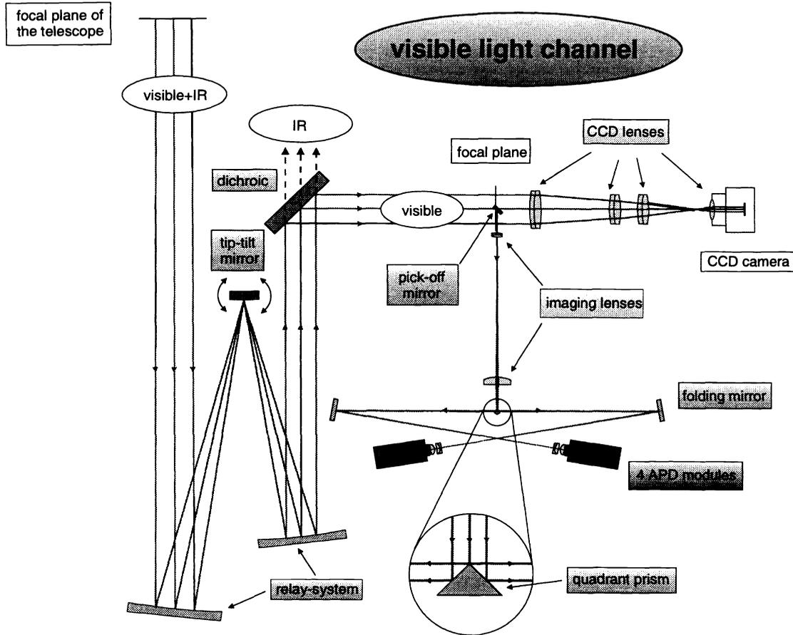
Figure 1: Schematic drawing of the optical layout of the visible light (sensing) channel of ROGUE. The shape of the quadrant prism is shown in the inset.
