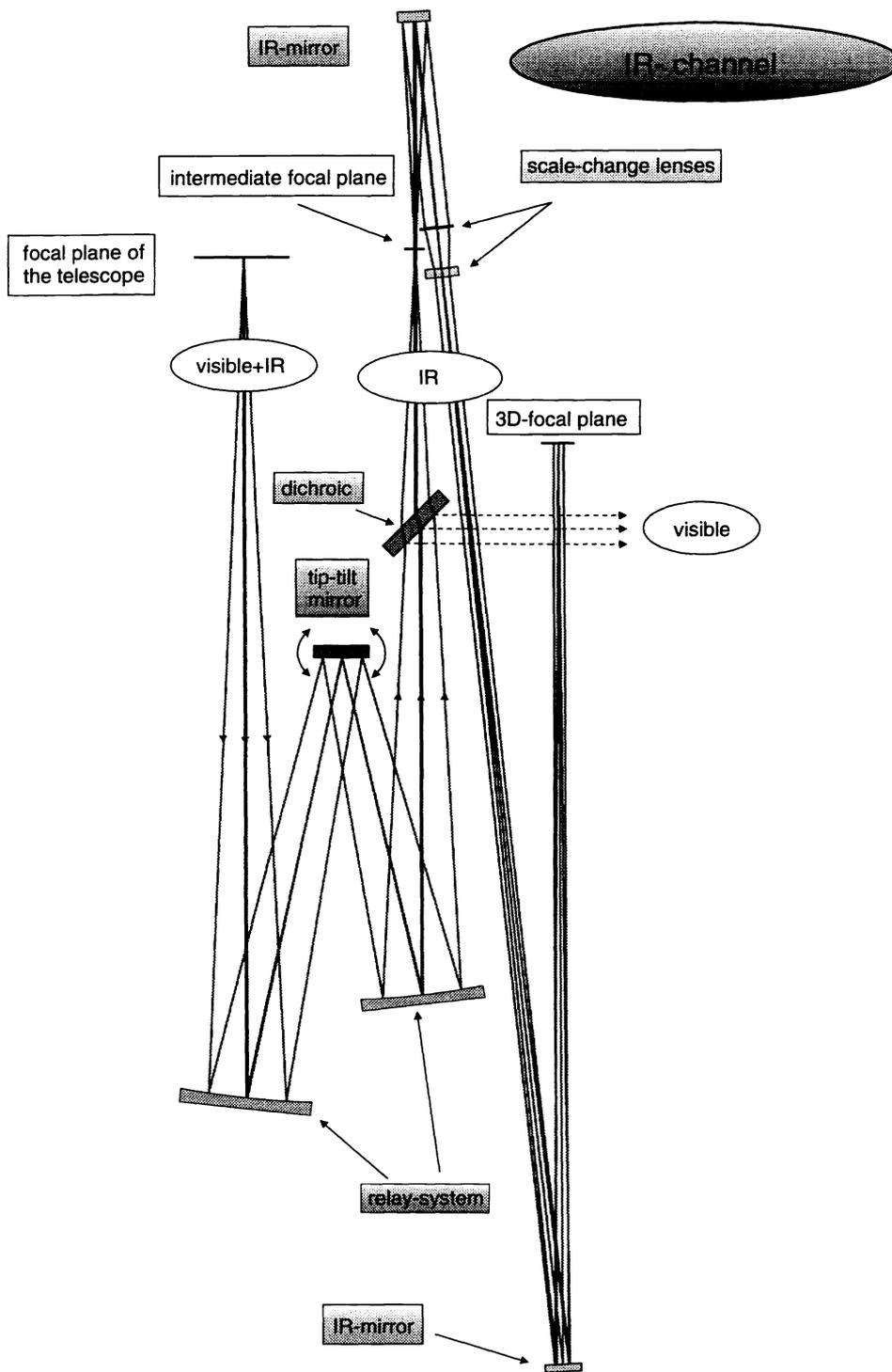
Figure 2: Schematic drawing of the infrared light path through ROGUE. The relay system and dichroic are the same elements as in Figure 1. Rays drawn are different from those in Figure 1.
