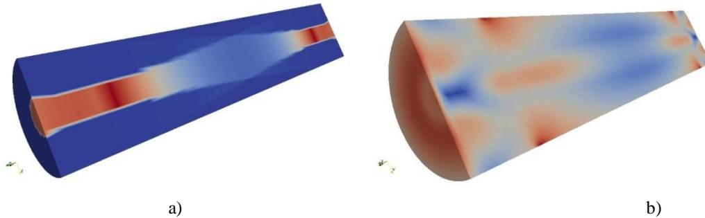
Figure 2. Nd:YAG crystal with doping of 0.3%, 0.4%, and 0.3% atn different sections. a) Population inversion b) Von Mises stress.
