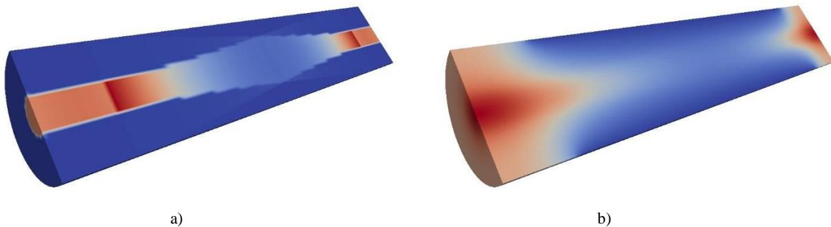
Figure 1. Nd:YAG crystal with doping concentration of 0.3%, 0.4%, and 0.3% at different sections. a) Absorbed pump power in laser crystal, b) Resulting temperature distribution.
