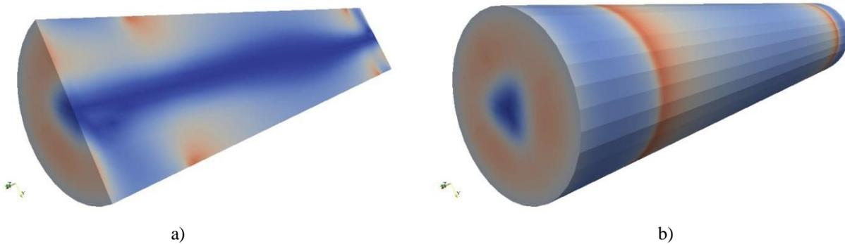
Figure 3. Nd:YAG crystal with doping 0.3%, 0.4%, and 0.3% in different sections. Birefringence for 111-cut.
