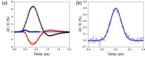
Fig. 4. (a) BD (circles) measurements of  $CS_2$  about zero delay with (curves) fits for (black) parallel, (red) perpendicular, and (blue) magic angle polarizations. (b) Zoomed in measurement at the magic angle. Taken from Ref. [6].
