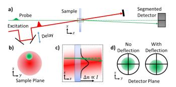
Fig. 1. a) Schematic diagram of beam deflection experiment, b) irradiance distribution of excitation (red) and probe (green) at sample plane, c) zoom in of a) at sample showing profile of  $\Delta n$ , d) probe beam on segmented detector without and with deflection. Figure taken from Ref. [4].
