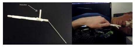
Figure 11 Tracking of a pen-shaped tool with an extension [30].
