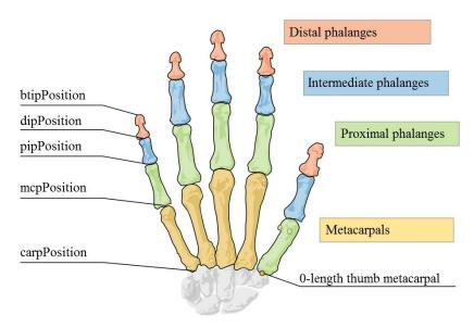
Figure 5 LEAP motion SDK: Skeletal tracking model [25].
