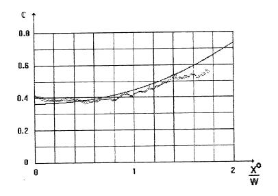
Fig. 6. Dependence of speckle contrast on observation point coordinate.
