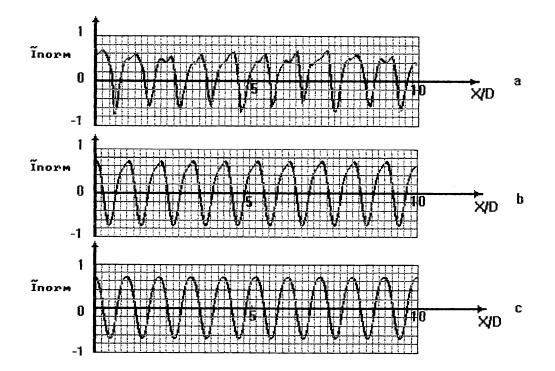
Fig. 3. The plot of dependence of alternate component of temporal intensity fluctuation of a scattered field (normalized on a maximal value) on waist beam center coordinate. The beam scans the surface having harmonic relief.
