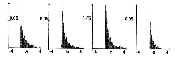
Fig.2. Histograms for probability density function of scattered intensity fluctuations at focused speckles diffraction from a rough surface. Values of intensity are normalized to that ones with zero mean and the unit standard deviation. Case of 4 speckles focused on the rough surface. W is a radius of the focused spot,  $W = 20\lambda$ ;  $W/L_c = 2$ ; a)  $\sigma_s = 0.001$ ; b)  $\sigma_s = 0.08$ ; c)  $\sigma_s = 0.1$ ; d)  $\sigma_s = 0.2$ .
