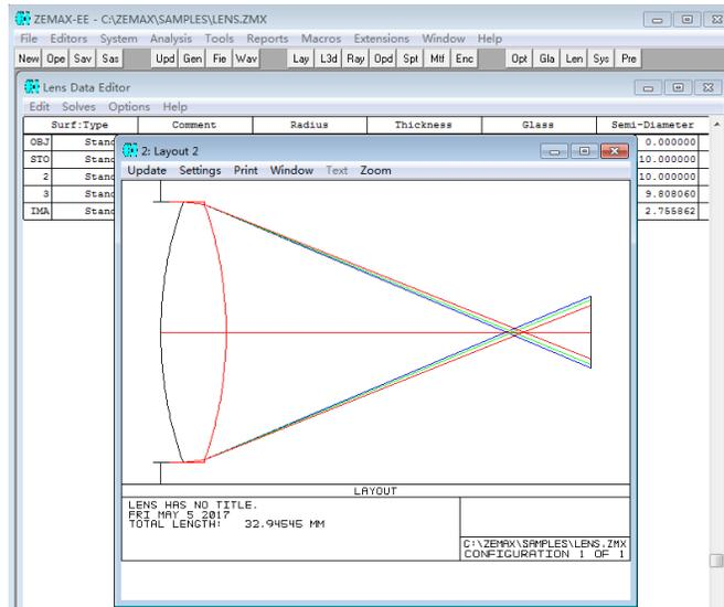
Figure 3. Light refraction by a lens illustrated using Zemax
