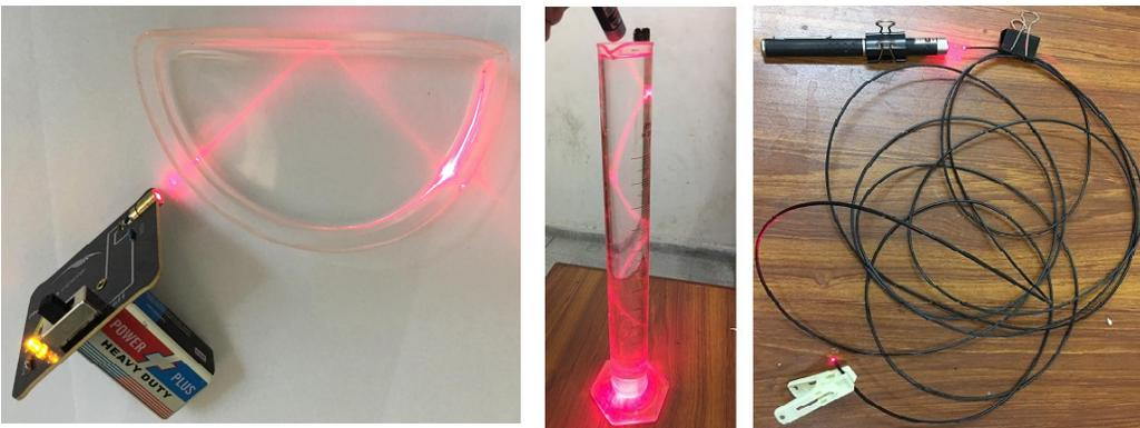
Figure 4. Total Internal Reflection of light from a) glass plate b) inside a water filled jar and c) through a fiber optics.
