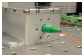
**Fig. 3.** Pump diode box.
