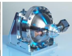
**Fig. 5.** Optical cavity assembly.
