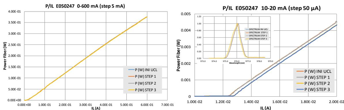
**Fig. 6.** L-I curves at initial, step 1, 2 and 3 of proton radiation for the MiniDIL PLM: (left) full driving current span of 0 - 600 mA and (right) zoomed area from 10 to 20 mA driving current. The inset shows the OSA trace at the various measurements points.
