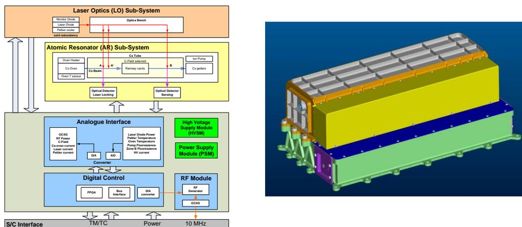
Fig. 1. Left: Functional Architecture of the optically pumped Cs clock, Right: View of the engineering model of the clock – below the housing of the electronics package (EP), above the atomic resonator (AR) and the laser and optics sub-system (L&O).
