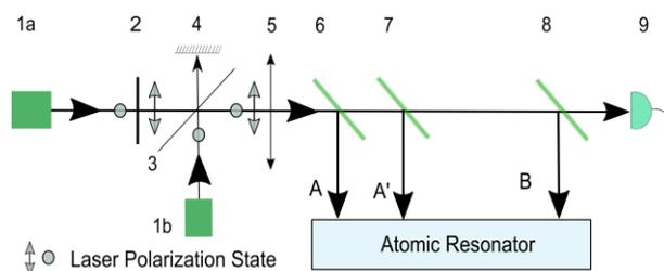
Fig. 2. Functional implementation of the Laser & Optics sub-system, with the components 1 Laser Diode, 2 waveplate, 3 polarizing beamsplitter, 4 beam absorber, 5 beam circularization, 6-8 beamsplitter, 9 photodetector for optical power detection.
