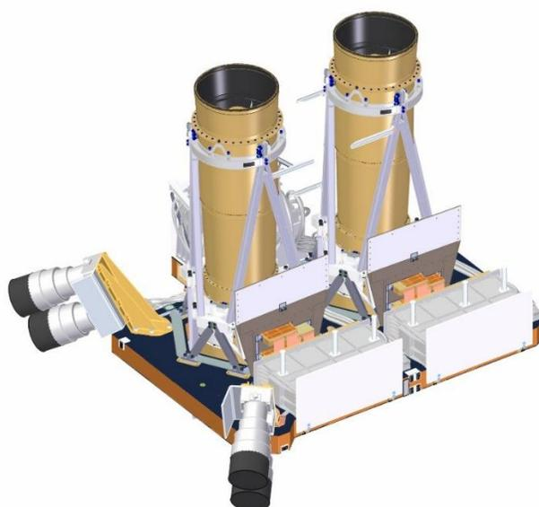
**Fig. 2.** 3D view of the Ingenio/SEOSAT primary payload
