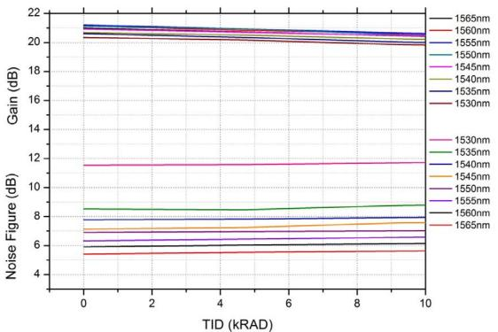
Fig. 4. EDFA-1 radiation test results: Gain and NF performance for 0-10 kRad TID.
