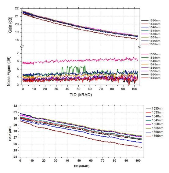
**Fig. 6.** Gain and NF performance of EDFA-2 from 0-100 kRad with 0 dBm input power (top) and with -10 dBm input power (bottom)
