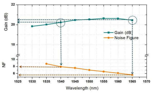
Fig. 5. EDFA-1 Gain and NF performance at 10 kRad TID with 0 dBm input power
