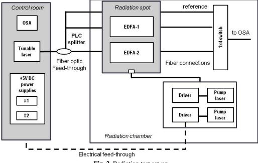
Fig. 2. Radiation test set-up
