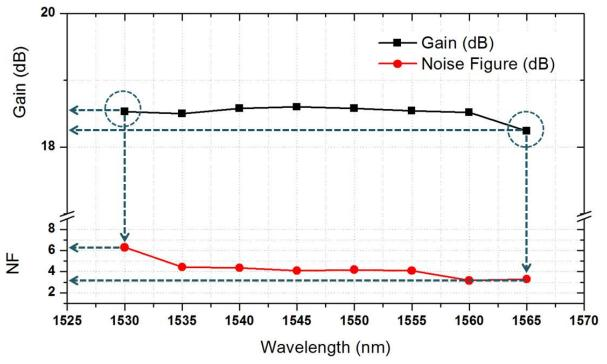
Fig. 7. EDFA-2 Gain and NF performance at 100 kRad TID with 0dBm input power
