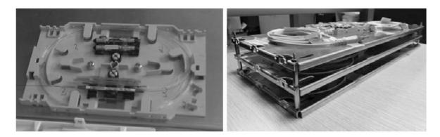
**Fig. 1.** Assembled EDFA optical engine under test (left) and EDFA optical engines mounted on Aluminum chassis suitable for transportation to the test-house (right)
