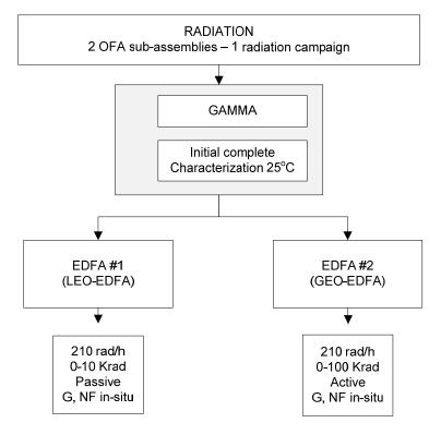
Fig. 3. Radiation test flow and conditions
