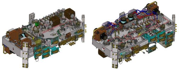
Fig. 4. Two sided optical bench, showing Oscillator side (left) and Amplifier/THG side (right)
