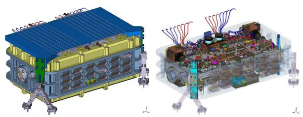
Fig. 1. FULAS pressurized housing with top-mounted cold plate and internal optical bench
