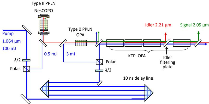
**Fig. 2.** Experimental set-up for the high energy MOPA. The wavelengths represented correspond to the case where the signal is emitted in the CO<sub>2</sub> R30 line around 2051 nm.
