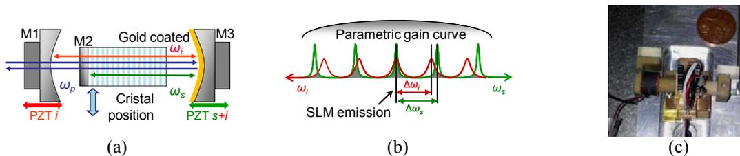
**Fig. 1.** (a) Schematic representation of the NesCOPO configuration, (b) mode overlapping between signal and idler cavities, SLM emission is achieved for one single exact coincidence within the parametric gain bandwidth, (c) picture of an integrated NesCOPO device.
