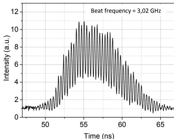
**Fig. 6.** Visualization of the instantaneous beat note between output pulses from the emitter and a DFB laser diode at 2051 nm on a fast oscilloscope.
