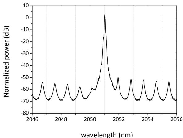
**Fig. 5.** Emission spectrum of the diode laser used as a spectral reference for beat note mixing and analysis. The measurement realized with an optical spectrum analyser.
