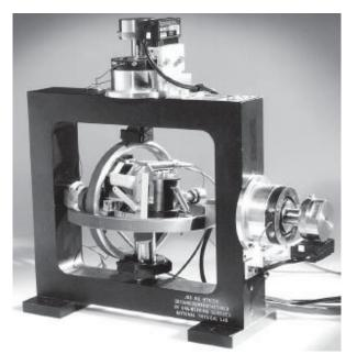
Fig. 1: The measuring station for the multi-lateration system.
