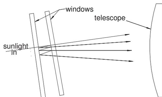
Figure 4-1 Ratioing method using windows
