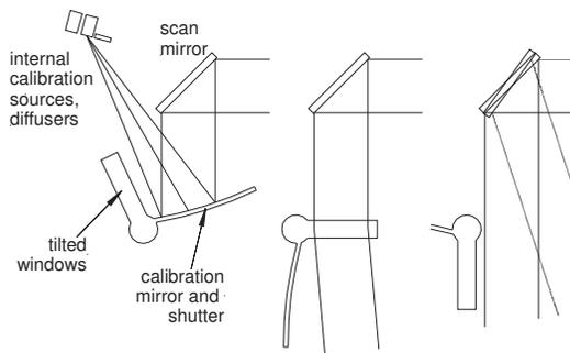
Figure 4-3 Deployment of separate components for absolute calibration and flat fielding
