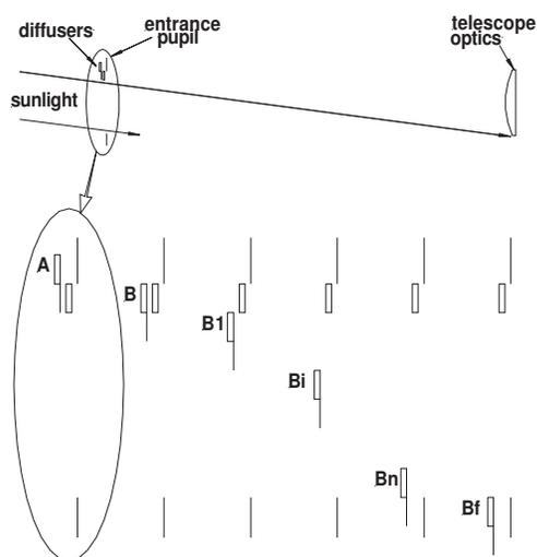
Figure 3-1 Ratioing method using 2 diffusers
