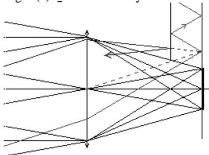
Fig. 1(d). Trapping of  $r$  and rejection of a ray entering parallel to  $r$  (on the top)
