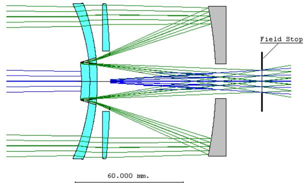
Fig. 3. Maksutov objective and field stop for a navigation camera.
