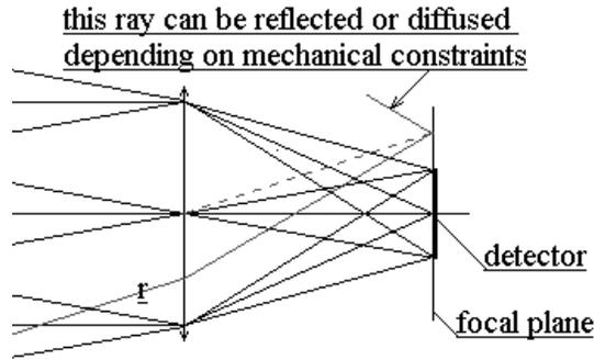
Fig. 1(a). First order ray tracing layout of the spatial filtering concept. The skew ray  $r$  is reflected by a flat focal plane.
