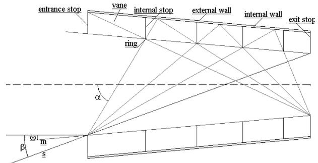
Fig. 2. A typical baffle design
