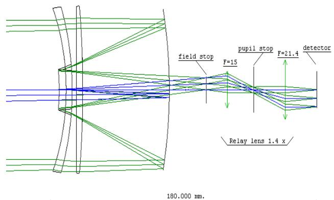
Fig. 4. Overall layout with a first order relay.
