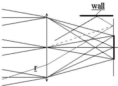
Fig. 1(b). First order ray tracing layout of the ray  $r$  reflected by a lateral wall after reflection on the insensitive area of the detector.
