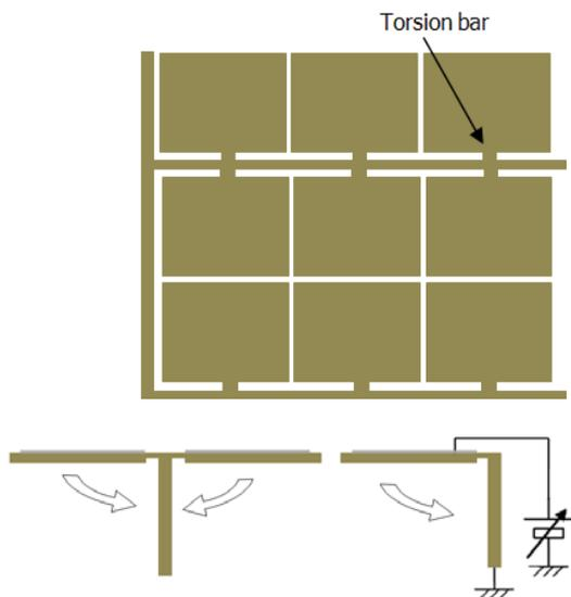
Figure 1 – MSA top view (top) and side view (bottom) of a section of the micro shutter array.
