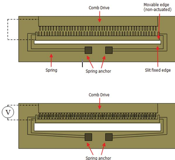
Figure 4 – Top view of the MEMS variable slit. Non-actuated position (top) and actuated position (bottom).
