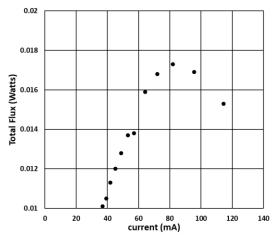
Figure 3. Total flux output from a white light LED as a function of drive current, up to and beyond the 35 mA rated forward current.
