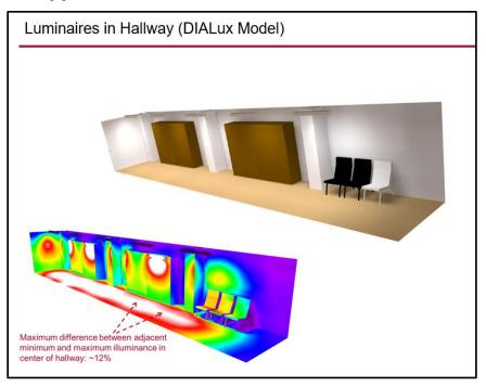
Figure 6 – Example of a page from a student's design report of a new hallway lighting arrangement showing a rendering from a DIALux model showing a rendering of the hallway and a pseudo-color map of the illumination levels predicted by the design.
