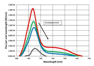
Figure 2. Four spectral scans of white light LED for drive currents of 82 mA, 95 mA, 115 mA, and 125 mA. The rated forward current is 35 mA.
