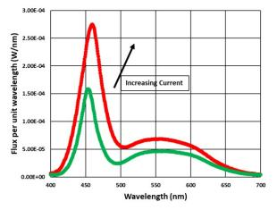
Figure 1. Spectra of white light LED for two currents below the rated forward current of 35 mA.
