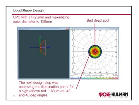
Figure 7 – Example of a page from a student's design report describing one of the interim steps in the design process of a luminaire and illustrating output from the optical design program LucidShape.
