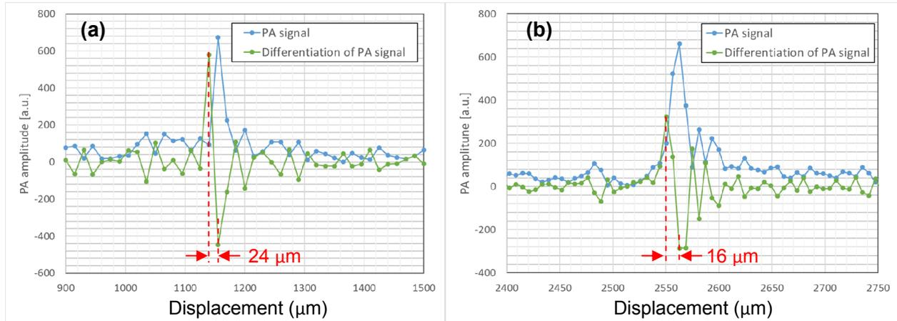
Figure 3. Graphs showing (a) horizontal resolution and (b) axial resolution
