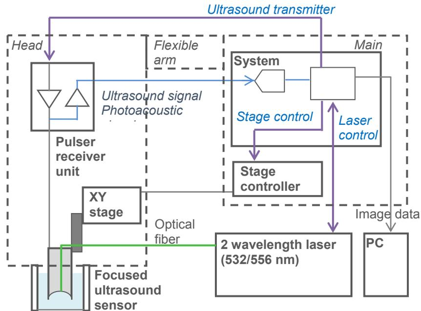
Figure 1. Block diagram of the HFUS-PAM system with dual-wavelength light sources
