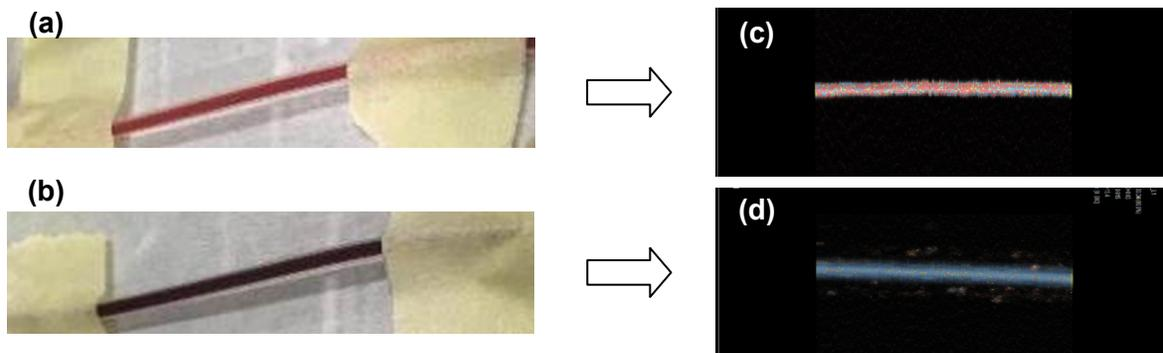
Figure 4. Appearance of the tube phantom (a) with intact horse blood, (b) with reduced horse blood, calculated oxygen saturation of the tube phantom (c) with intact horse blood, (d) with reduced horse blood measured with HFUS-PAM
