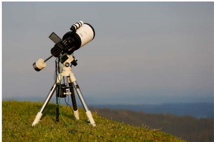
Figure 4: Telescope on computerized mount with camera
