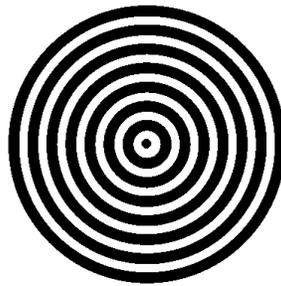
Figure 8. Rings structure for a calibration target
