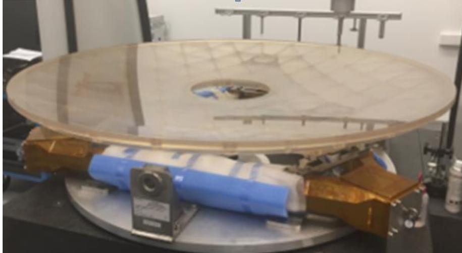
Figure 7. M1 Mirror on instrument Si<sub>3</sub>N<sub>4</sub> main frame. This 1,5 m Zerodur mirror has a total mass around 25 Kg/m<sup>2</sup>.
