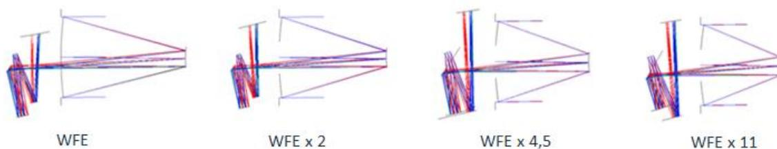
Figure 2. Effect of the instrument volume on its performance: the more compact, the more degradation appears due to any misalignment
