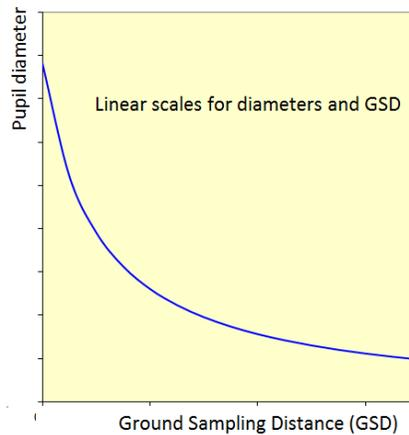
Figure 1. Entrance pupil evolution with respect to the ground sampling distance for a given orbit and for a given MTF performance. Improvement in GSD can affect significantly the entrance pupil size.
