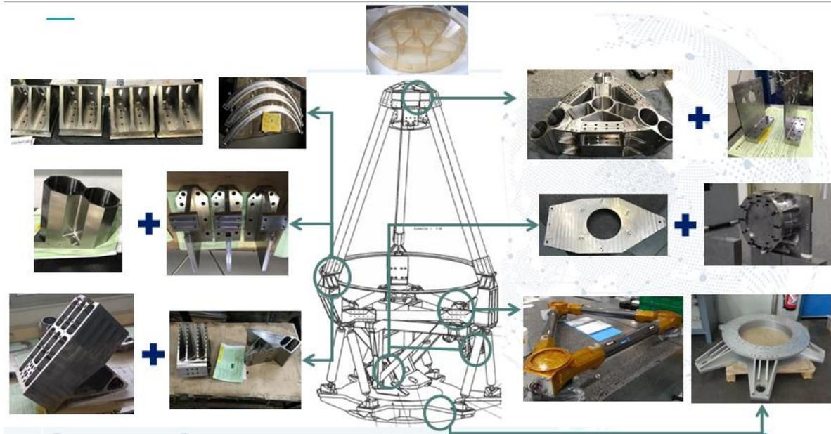
Figure 11. Manufacturing of the active observation instrument full scale demonstrator in progress at Thales Alenia Space. It will allow to demonstrate the performance of the control loop to validate in full scale the efficiency of all developed technologies for active optics.
