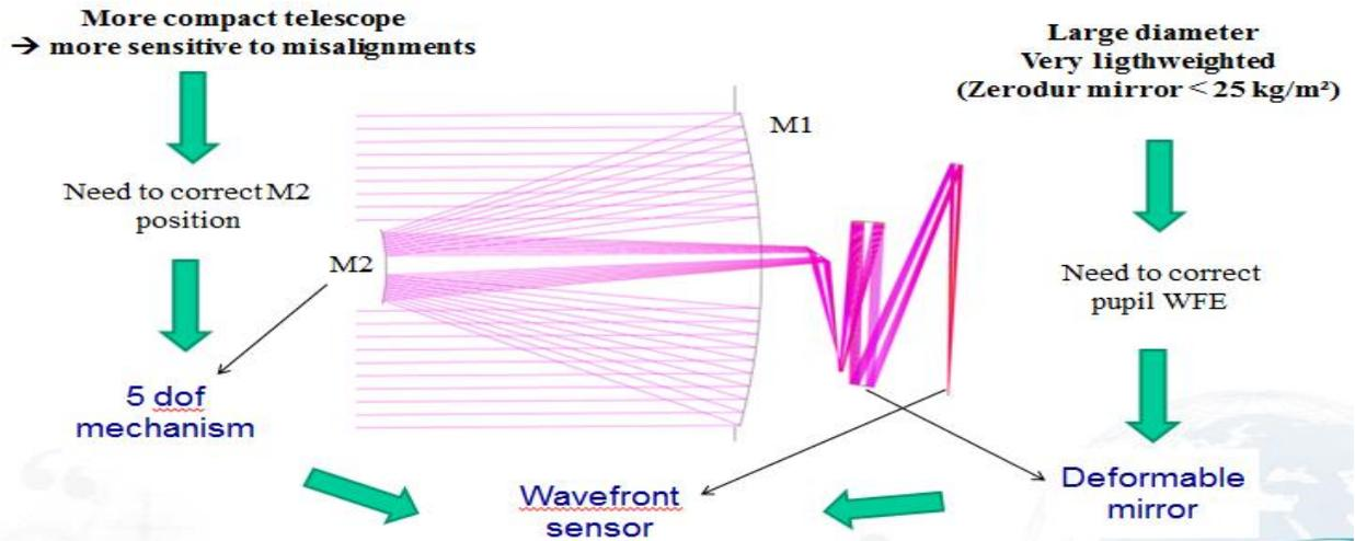
Figure 5. Implementation of active optics proposed in the frame of TANGO project for the next generation of space telescope for Earth observation
