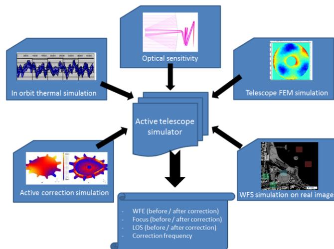
Figure 6. A end-to-end simulator for the active control loop has been proposed to assess the final added value of active optics and specify the needed requirements associated to active components (amplitude, accuracy, working frequency)
