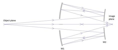
Figure 5. Flat image anastigmat relay
