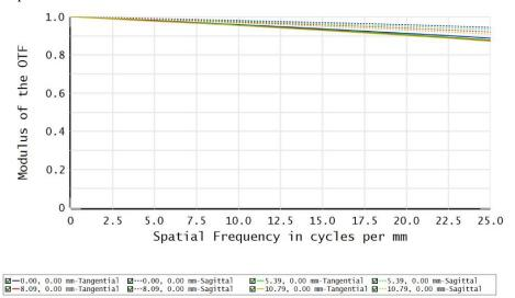
Figure 7. MTF plot for the central wavelength (650 nm) considering pixel size of 20 µm (Nyquist frequency 25 cycles/mm)
