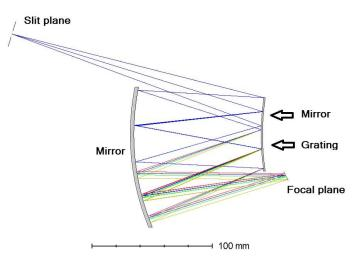
Figure 6. Spectrometer layout
