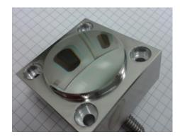
Figure 4. The Freeform convex grating. Credit AMOS.
