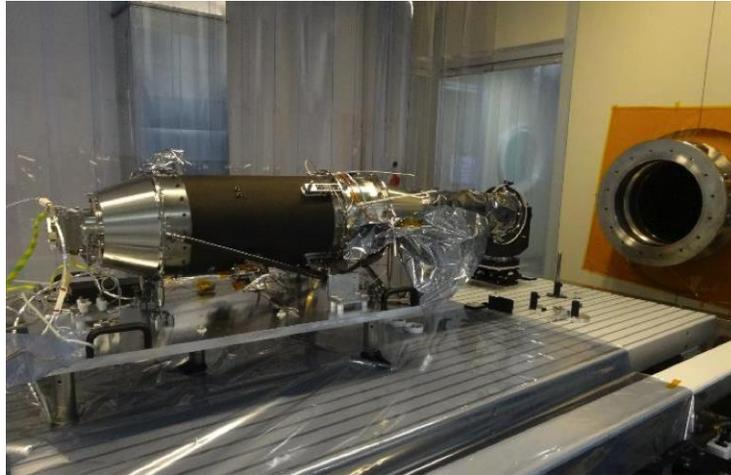
Figure 5: Metis on the SPOCC optical bench.
