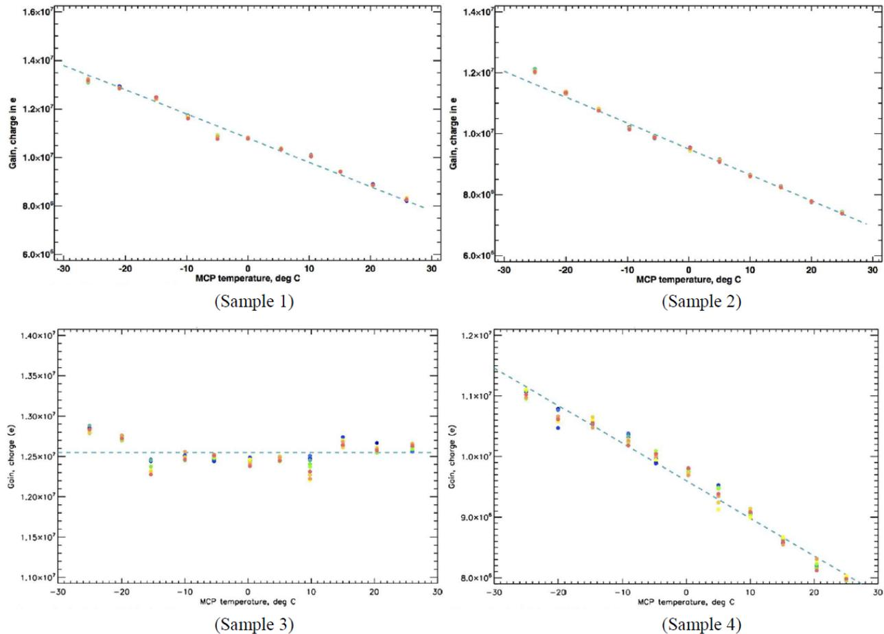
Figure 6. Variation of the gain of four samples of MCPs as a function of temperature. Each sample is taken from different batches. Samples 1 and 2 are from PHOTONIS USA and sample 3 and 4 from PHOTONIS France.
