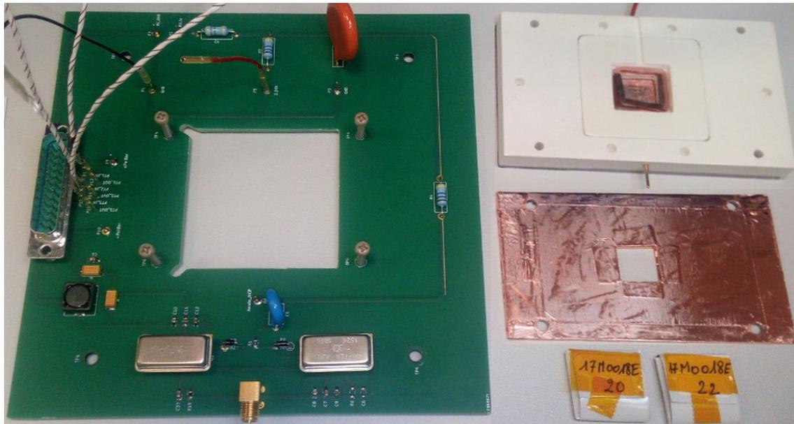
Figure 4. View of the setup parts showing the front-end electronic board, the ceramics, the grounding plate and the MCP samples.
