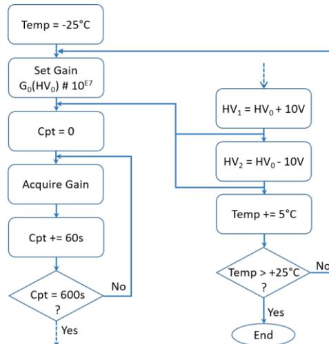
Figure 2. Procedure implemented in order to acquire the gain of the MCP chevrons.
