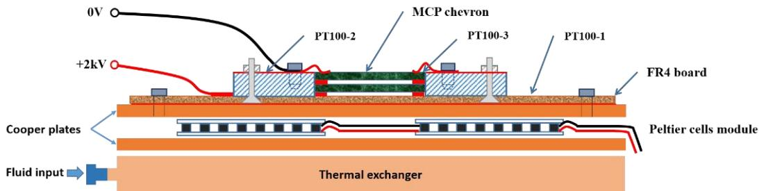
Figure 1. Setup used for measuring the resistance of the MCP chevrons.
