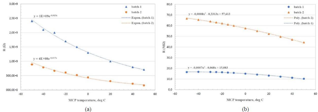
Figure 5. Variation of the resistance versus temperature of four MCP chevrons taken from two different batches. The plot (a) represents data from MCP samples 18x18 mm<sup>2</sup> and the plot (b) data from full-size MCPs 58x90 and 48x140 mm<sup>2</sup>.
