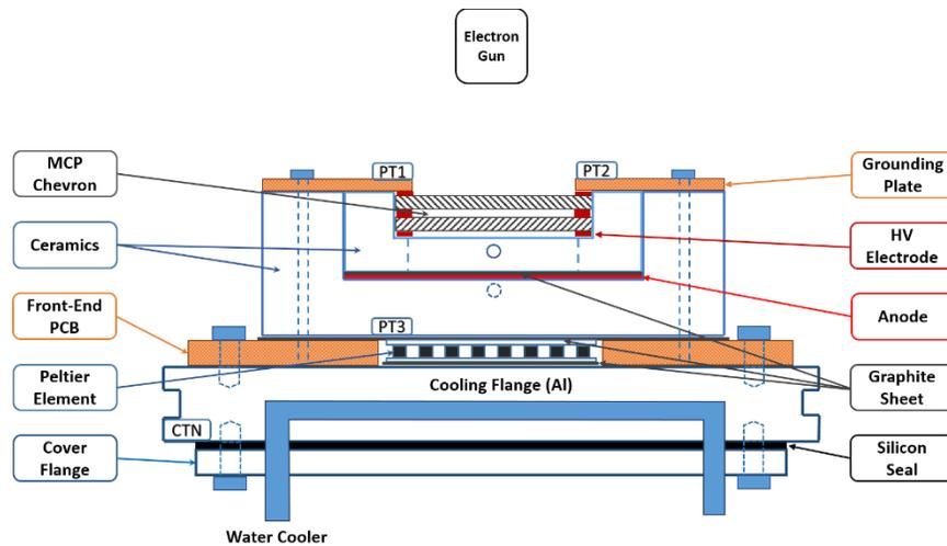
Figure 3. Setup used for measuring the gain of the MCP chevrons.
