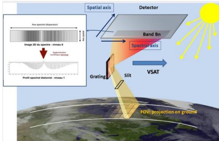
Figure 2: MicroCarb instrument principle
