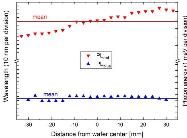
Figure 1. PL peak positions at different distances from the center of a 3” wafer in a 5×3” platen configuration.
