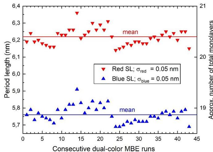
Figure 3. Period lengths of both SLs for consecutive dual color structures. The right axis indicates the approximate sum of the GaSb, InAs and InSb monolayers.
