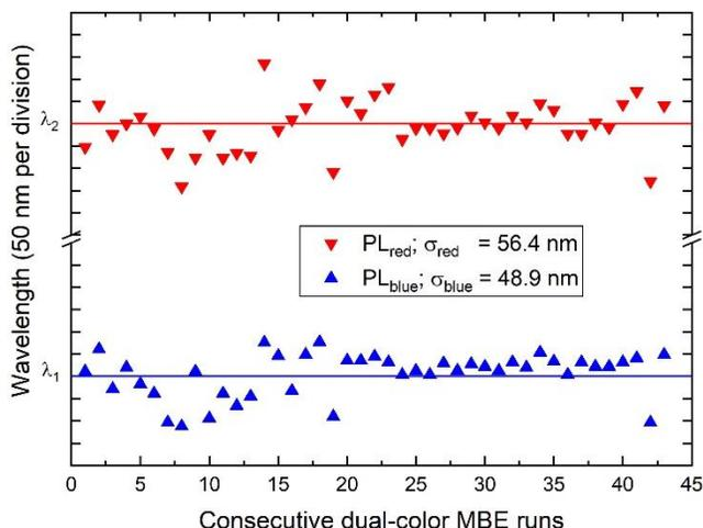
Figure 4. PL peak position for both SLs for consecutively grown dual color layer structures.
