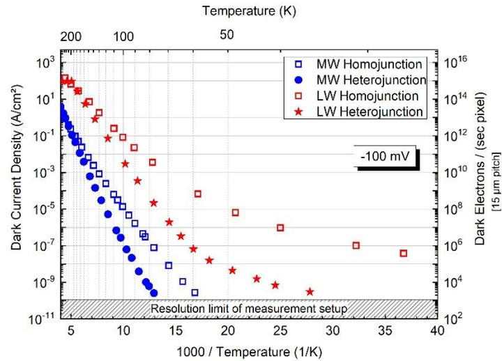
Figure 5. Temperature dependent dark current density of homo- and heterojunction T2SL devices at 100 mV reverse bias. The corresponding number of dark electrons per second per pixel normalized to 15  $\mu\text{m}$  pixels is shown on the right axis.
