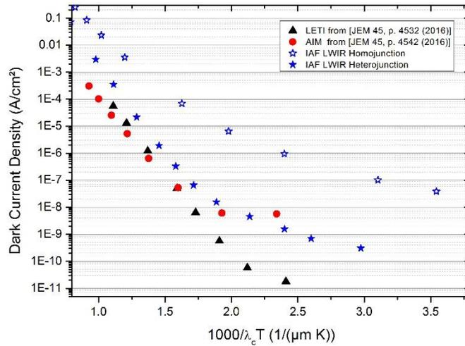
Figure 6. Dark current density of T2SL structures as a function of the inverse temperature and inverse cut-off wavelength in comparison with published HgCdTe data<sup>10-11</sup>.
