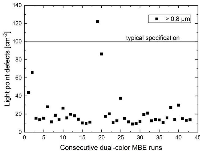
Figure 2. Density of light point defects sized between 0.8 μm and 10 μm measured with a Surfscan 6220 for consecutive growth of dual-color structures with more than 10,000 shutter movements per growth.
