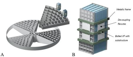
Fig. 6. (A) IXO Hierarchical concept assembly and (B) X-Ray Optical Unit
