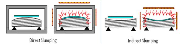
**Fig.1.** Schemes of the slumping techniques investigated in the present study: "direct" (left side) and "indirect" (right side) slumping techniques.
