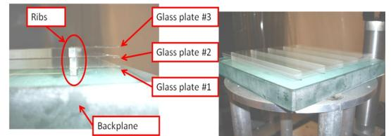
**Fig. 4.** Breadboard of three flat stacked plates developed during the Phase 1 of the project. The first foil is connected to a thick glass backplane.
