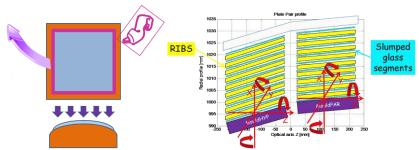
**Fig. 3.** Left side: with the use of the vacuum suction on the formed foil placed on the mould the shape after slumping is restored, correcting the errors due to the spring back after the detaching; in that way the foil can be easily handled during the integration. Right side: iterating the procedure it is possible to create an X-Ray Unit made of several pairs stacked together; for this purpose reinforcing ribs are used to connect each plate to the next one.
