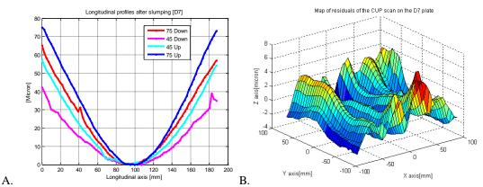
**Fig. 5.** (A) Longitudinal profiles of a slumped glass, produced via direct slumping foils, taken at +/-45mm and +/-75mm from the centre before the integration. (B) Map of the same sample after integration with ribs on a backplane. The corresponding angular resolution is 20 arcsec HEW.
