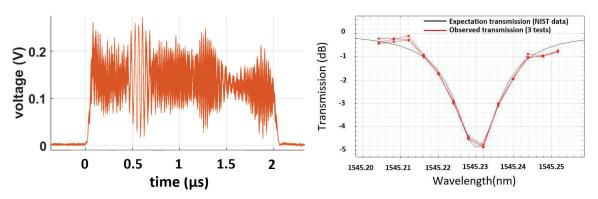
Figure 6 – Left: Time profile of a double-comb emitted pulse; Right: Measured transmission of the HCN line at 1545.23 nm in pulsed mode with 76µJ, 10 kHz, 2µs square-shaped pulses.
