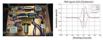
Figure 3 - Left: I/Q demodulation stage of the FMS-based stabilization loop. Right: Locking signals observed on channels I, Q, and Z.
