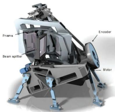
Figure 2. (left) sketch of the Mertz Interferometer (right) Mertz Interferometer design with Dual Swing Mechanism for IASI NG instrument
