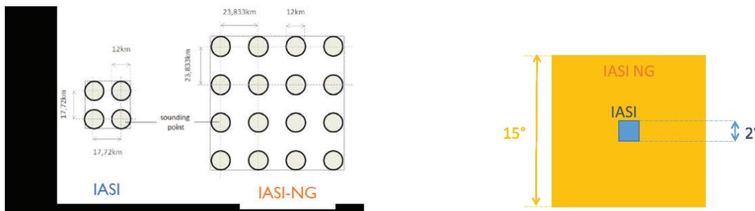
Figure 1. Scheme of the Field of regard on Earth (left) and inside the interferometer (right): IASI/IASI-NG comparison.
