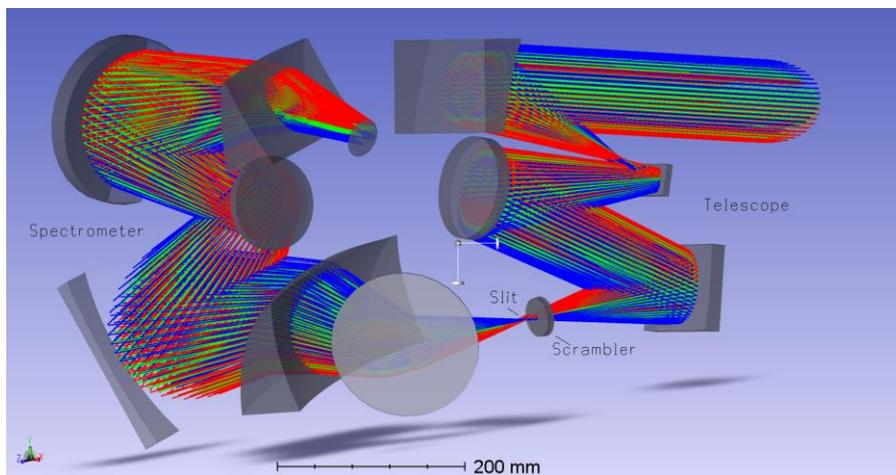
Figure 1: Full HIS optical design schematic
