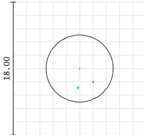
Figure 6: Illustration from a simplified paraxial 191 mm focal length system at 1500 nm wavelength where the prism are at 45 deg to each other. Airy's disc is given for reference
