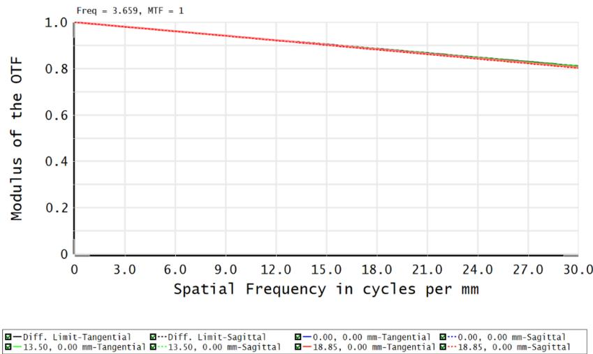
Figure 2: Optical MTF of a spectrometer only for some point on the slit at 1500nm. The sagittal curves are ACT and the tangential one ALT.
