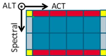
Figure 9: Detector axes: ACT, ALT and spectral
