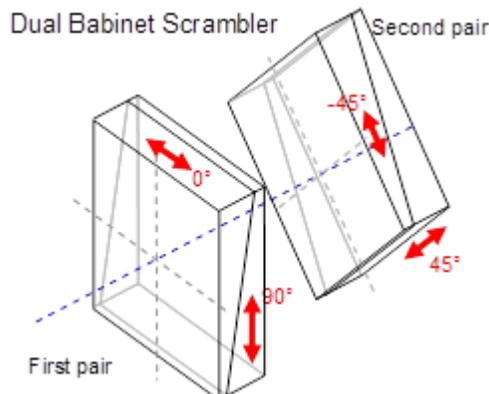
Figure 4: Schematic principle of a DBPD
