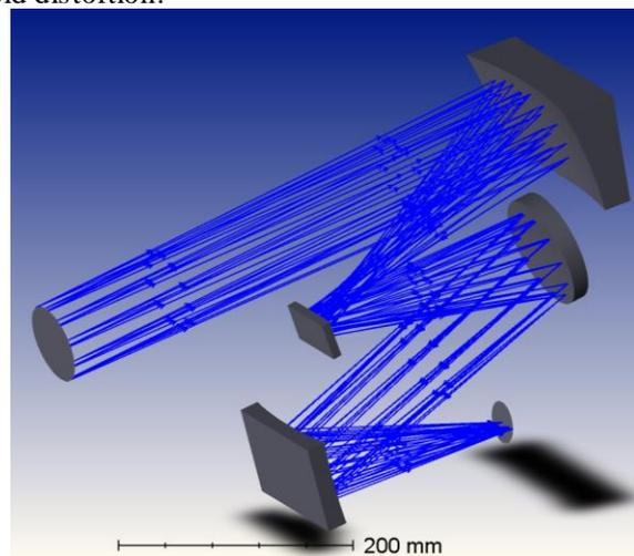
Figure 3: Optical layout of current telescope
