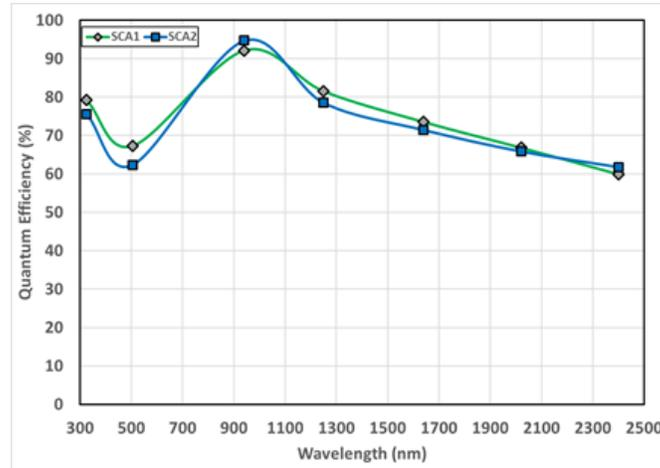
Figure 10: Tested quantum efficiency of new detector coating.
