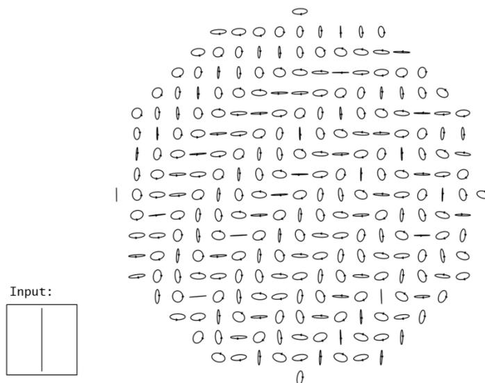
Figure 5: Polarisation pupil map at the rear surface of the last prism in the current baseline system.
