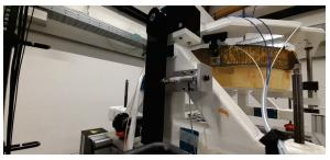
Figure 2. The TS sitting on the safety foam cushion. The yellow disk (coated with kapton) is the aluminum honeycomb RB. Please note the small air gap between the TS and the RB.
