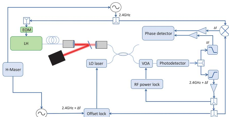
Figure 4: Setup for sideband phase noise measurement
