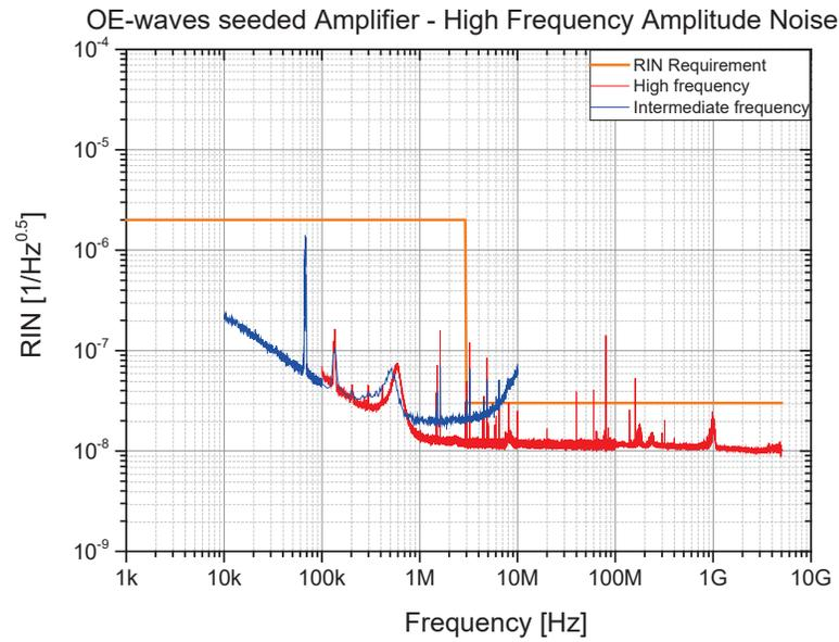
Figure 17: Power stability high frequency measured with CSEM LH BB with OEwaves seed laser
