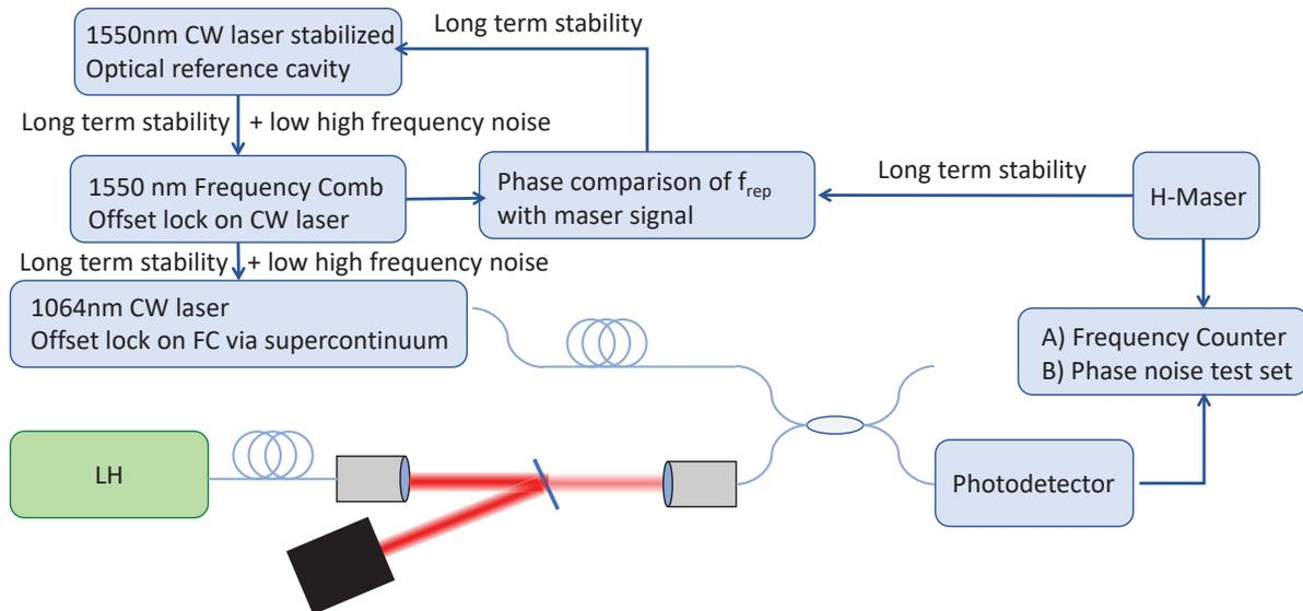
Figure 7: Architecture of frequency noise measurement setup for the [30  $\mu$ Hz; 3 kHz] frequency range.
