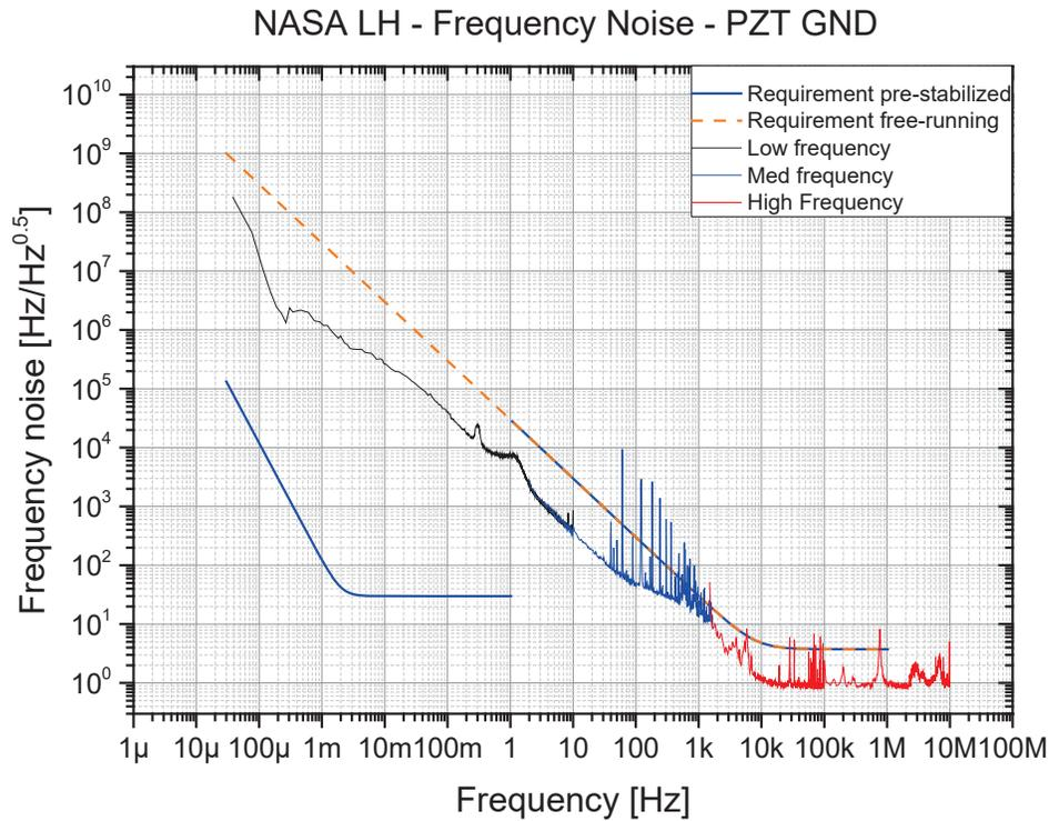
Figure 19: NASA LH piezo grounded frequency noise measurement (black / blue / red curve). Measurement (excepting spikes) is fully in specification.
