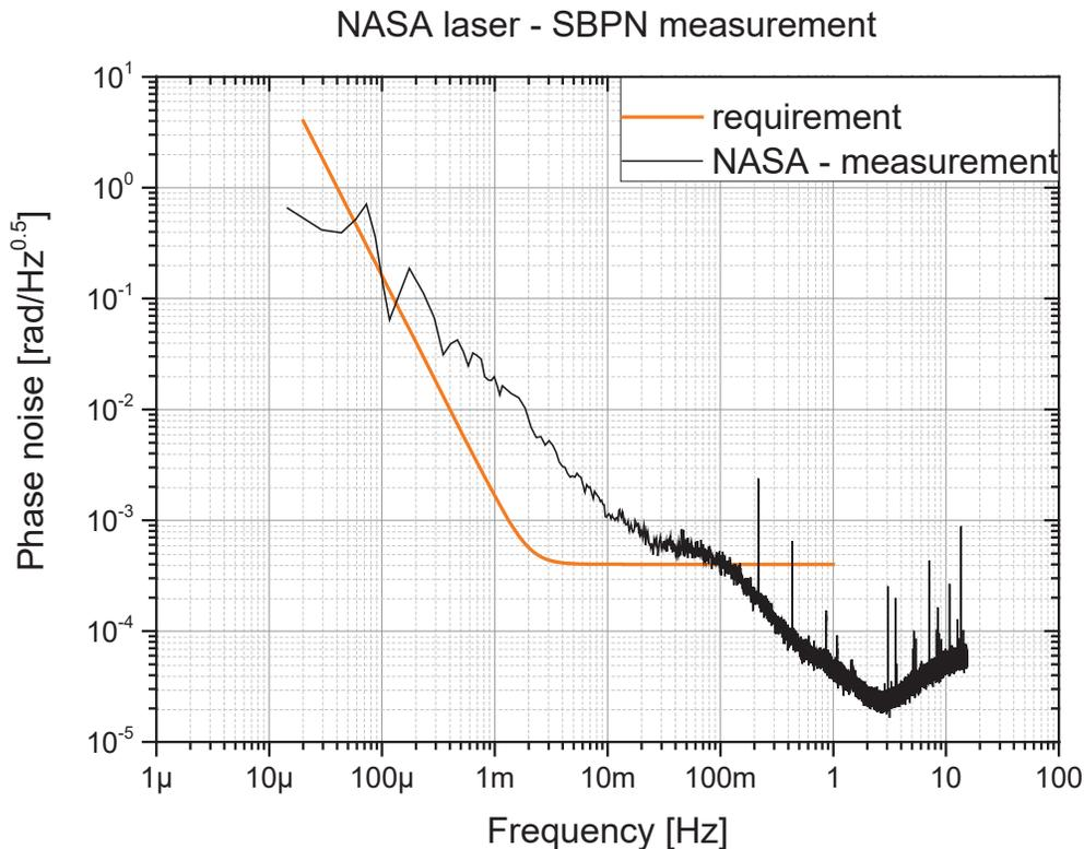
Figure 18: Measurement of the SBPN on the NASA laser
