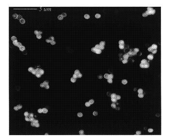
Figure 4. True color image of a mixture of CdSe/ZnS QD-tagged beads emitting singlecolor signals at 484, 508, 547, 575, and 611 nm. The beads were spread and immobilized on a polylysine-coated glass slide, which caused a slight clustering effect.
