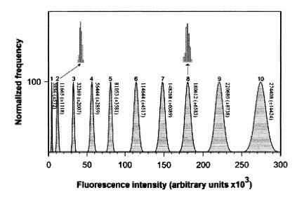
Figure 5. Spectroscopic analysis of single-bead fluorescence intensities. Each histogram plots is corresponding to one of the ten intensity levels, derived from 100-200 measurements. On the right side of each curve is shown the average fluorescence intensity as well as the standard deviation (in parentheses). Representative raw data are shown for levels 2 and 8.
