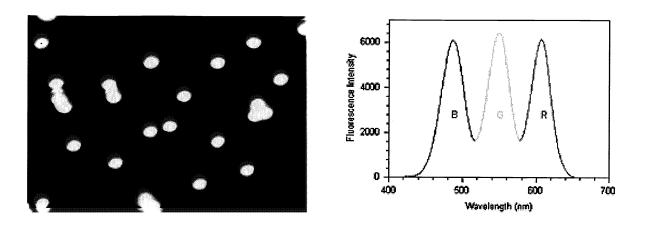
Figure 6. Triple color QD-tagged beads with precisely controlled fluorescence intensities. (Left) Fluorescence image of color-balanced beads. (Right) Single-bead fluorescence spectrum, showing three separated peaks (484, 547, and 608 nm) with nearly equal intensities.
