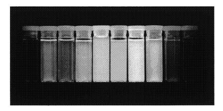
Figure. 2. True color fluorescent image of a series of ZnS-capped CdSe QDs, simultaneously excited with a handheld UV lamp. The colors are clearly distinguishable one from another.
