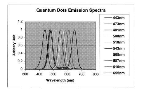
Figure 3. Size-dependent fluorescence spectra corresponding to the samples shown in Figure 2.
