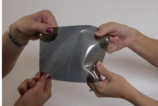
**Figure 2. Flexible Metal Rubber™ Nanocomposite Material.**
