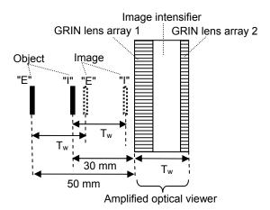
Fig. 5: Experiment using amplified optical viewer (side view). Objects I and E are letters both with 32-point font. I is 30 mm from array 1 and and E is 50 mm from same array. Center of both letters is offset 6 mm horizontally. Both images are separated from two object positions by Tw (45.5 mm), i.e., thickness of amplified optical viewer.
