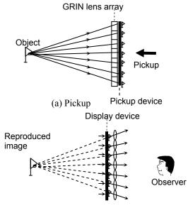
(b) Display (correct depth) Fig. 2: Integral method with orthoscopic image
