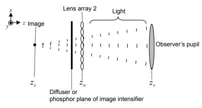
Fig. 7: Reproduced image behind exit plane of optical viewer
