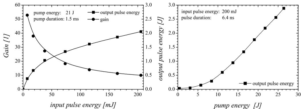
Figure 6. Nanosecond pulse amplification, pulse duration:  $6.4 \text{ ns}$ , numbers of passes: 4; (a) Output pulse energy and total gain vs. input pulse energy at a pump energy of 21 J, (b) Output pulse energy vs. pump pulse energy, input pulse energy: 200 mJ.
