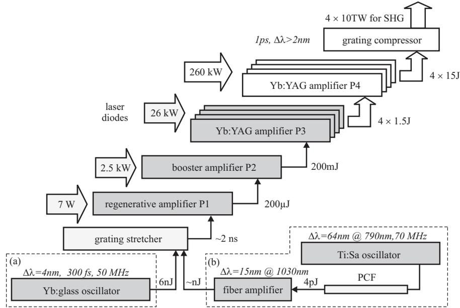
Figure 1. Outline of the PFS pump laser system, four-stage diode-pumped chirped-pulse amplifier chain, preliminarily seeded by front-end (a), Later, a broadband Ti:Sa oscillator serves as common front-end (b) for both OPCPA-chain and the pump laser, PCF: photonic crystal fiber for shifting the center-wavelength of the seed-pulses from 790 nm to 1030 nm.
