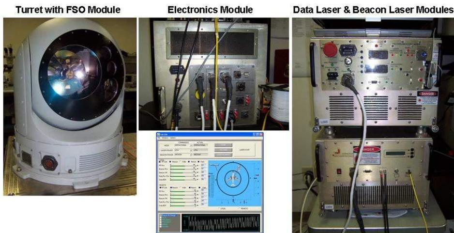
Figure 4, Laser Communications System utilizing MX-12 Turret
