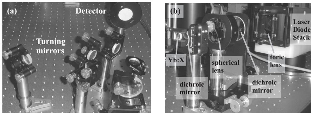
Figure 6. Experimental setup of the Yb-based diode-pumped multi-pass amplifier.
