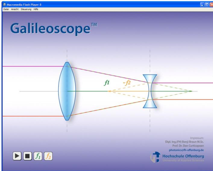
Figure 16a: Galileoscope™, optical path
