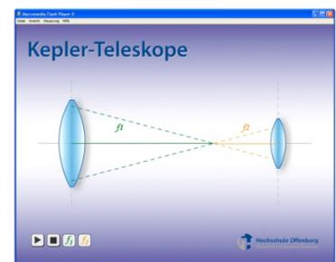
Figure 17b: Kepler Telescope, lens geometry
