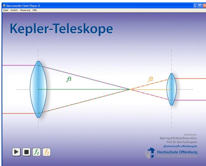
Figure 17a: Kepler Telescope, optical path
