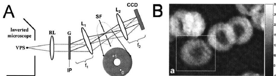
Figure 2. (A) Schematic of a diffraction phase microscope and (B) a quantitative phase image of red blood cells<sup>10</sup>.
