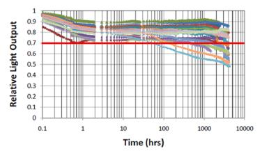
Figure 4. Relative light output over time for 22 LED-based replacement A-19 lamps<sup>[11]</sup>
