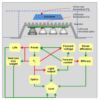
Figure 2. Simple schematic of a lighting system and decision chart for optimizing system performance<sup>[11]</sup>
