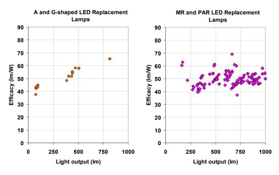
Figure 1. Plotted light output and efficacy of LED replacement lamps (A, G, MR, and PAR types) qualifying for the Energy Star program logo (based on data from the Energy Star website, August 2011)<sup>[10]</sup>
