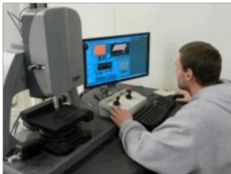
Figure 8 – Student working with Zygo MetroPro software and white light profilometer.
