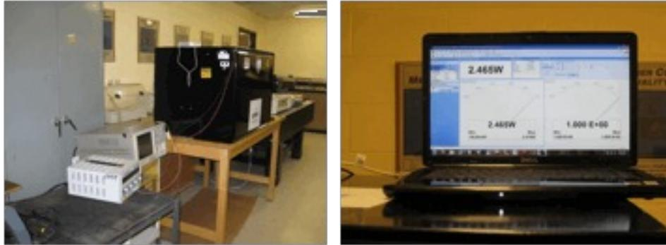
Figure 4 – (Left) Unit under test. (Right) Ophir StarLab software interfaced with LabView for measuring laser
