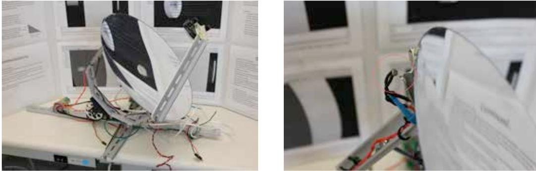
Figure 6 – Revised version of the solar tracker/collector using a lightweight Cassegrain mirror system. Left: Mirror assembly with motor to the left. Right: Light sensors are mounted below the rim of the mirror on opposite sides.
