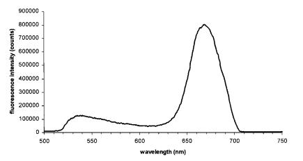
Fig. 3 Emission spectrum of Cy5 after excitation with the short pulsed diode laser (398 nm).
