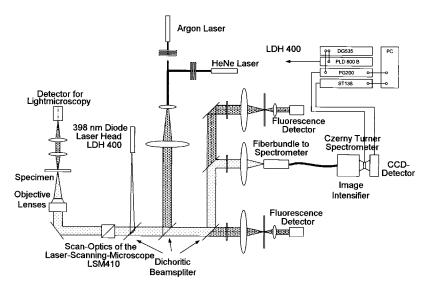
Fig. 1 Experimental setup for laser scanning microscopy and time-resolved microspectrofluorometry.
