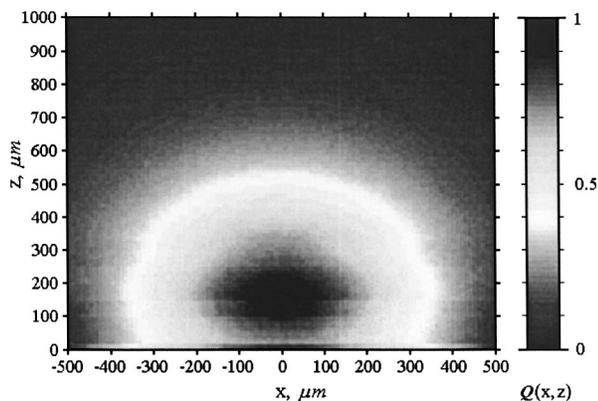
**Fig. 5** Two-dimensional distributions of the spatial depth sensitivity  $Q(x,z)$ . The optical parameters of skin layers were chosen for 488 nm (Table 1). The fraction of fluorescence that is sensitive to sensor and topical dermal layers is close to one another. The diameter and numerical aperture of the detector are equal to 1000  $\mu\text{m}$  and 0.63; acceptance angle  $\theta_d = \sin^{-1}(NA/n_0)$  is 40° with NA the numerical aperture.
