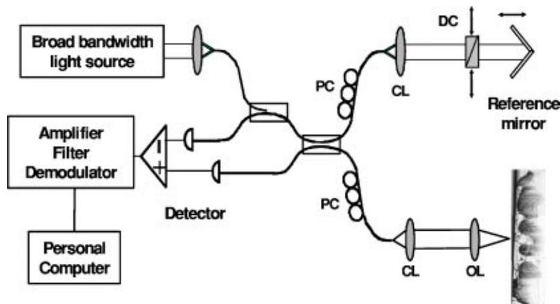
**Fig. 1** Schematic of a fiber-based UHR OCT system: CL, collimating lens; OL, objective lens; DC, dispersion compensation unit; PC, polarization controllers.
