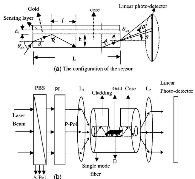
**Fig. 1** (a) Configuration of the sensor. (b) Beam coupled in and out of the D-type optical fiber biosensor (PBS, polarization beam splitter; PL, polarizer).
