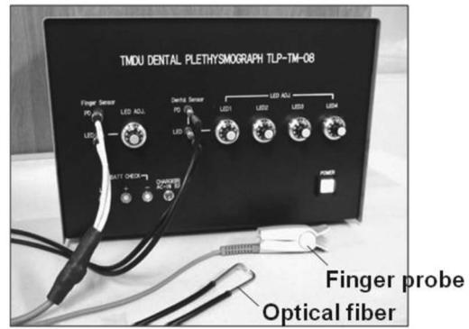
**Fig. 2** Multiwavelength optical plethysmograph.
